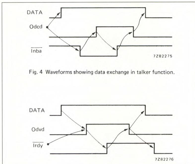
Fig. 4 Waveforms showing data exchange in talker function.
